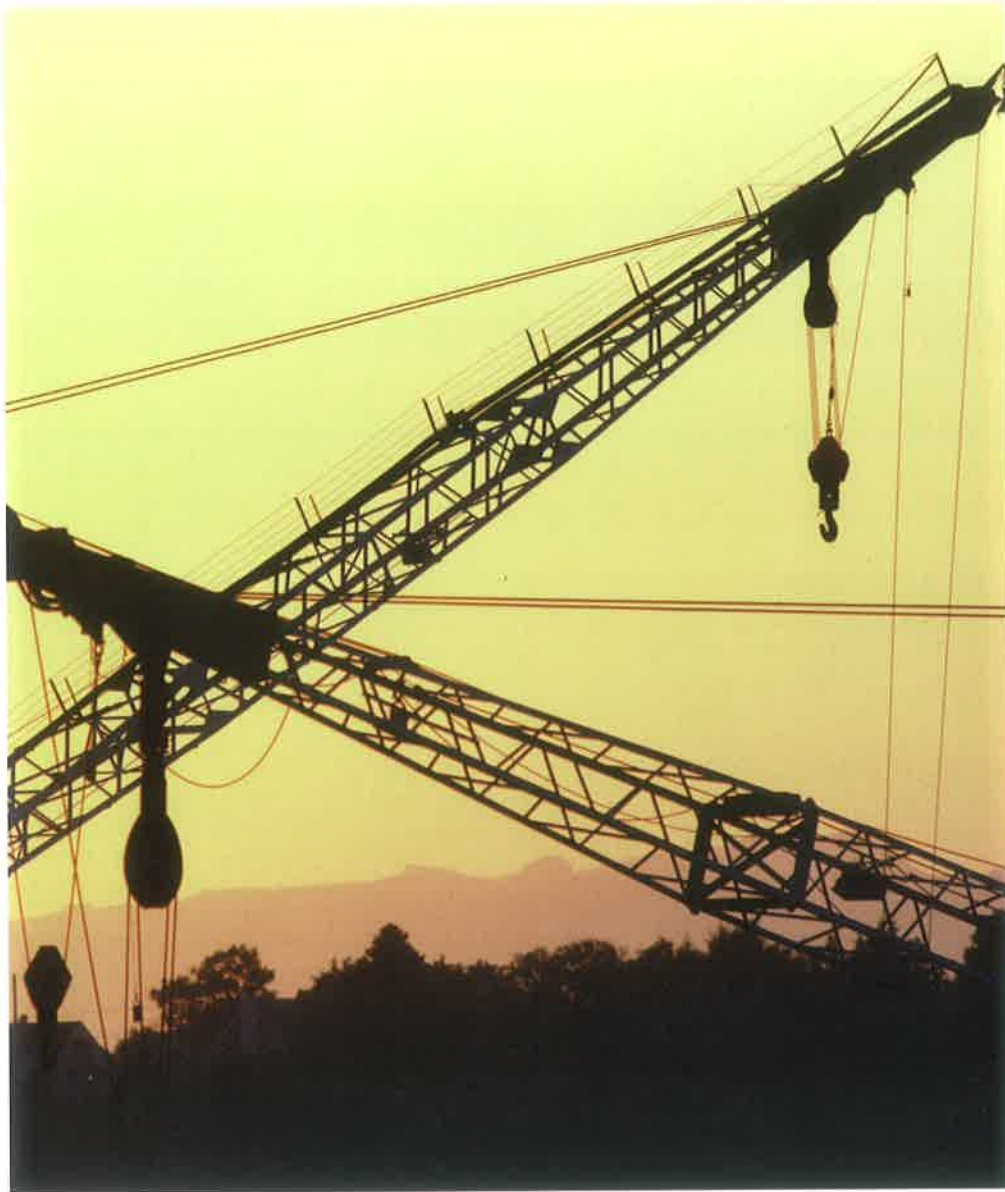
Large cranes use compound pulleys to lift heavy loads.
