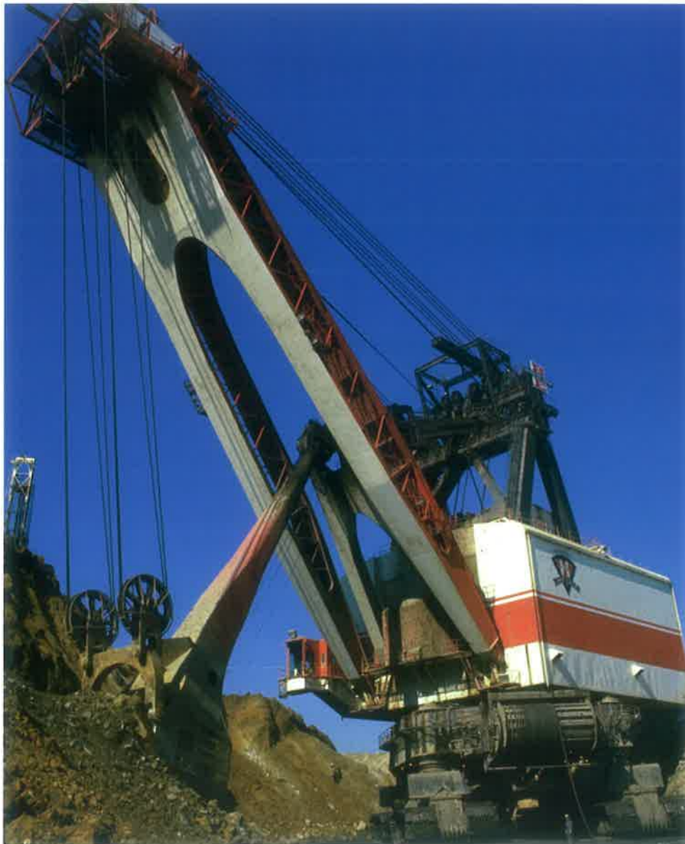
This enormous power shovel uses pulleys to move huge quantities of earth at a mine in Hanna, Ohio.
