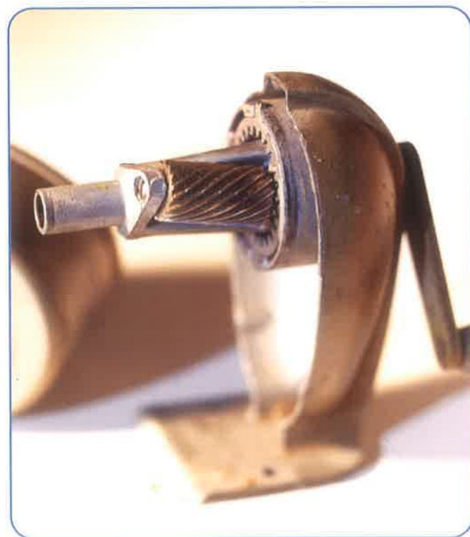
▲ Figure 35 A pencil sharpener is an example of a compound machine that we see every day. It contains several simple machines that work together.
