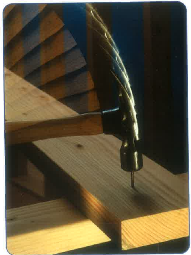
▲ Figure 20 The hammer exerts a force on the nail and the nail exerts an equal and opposite force on the hammer. However, the nail accelerates more than the hammer does because the nail has a smaller mass.
