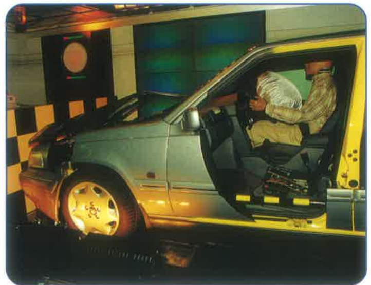
▲ Figure 17 Inertia causes a test dummy to keep moving forward when the car stops suddenly. The seat belt and air bag keep the test dummy "driver" from hitting the steering wheel or windshield.
