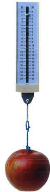
▲ Figure 4 The spring scale shows that the force needed to lift the apple is 1 newton.
