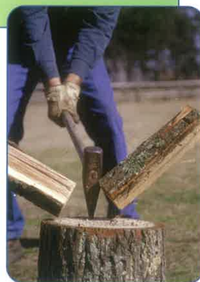
► Figure 26 An ax is a wedge that can be used to chop logs for firewood. A downward input force is transferred to a sideways output force that splits a piece of wood in half.
